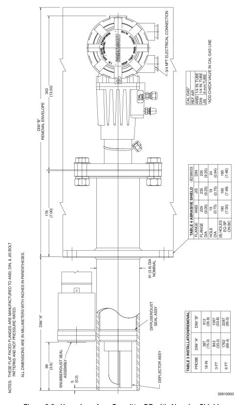
Figure 2-2. Hazardous Area Oxymitter DR with Abrasive Shield
